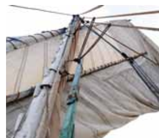
The sails are reefed by hauling in on the clewline
